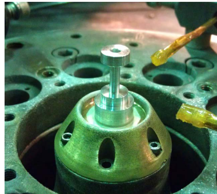
Z-scale liners, aluminum (150 \mu m thick, 3mm OD and 10mm tall)
