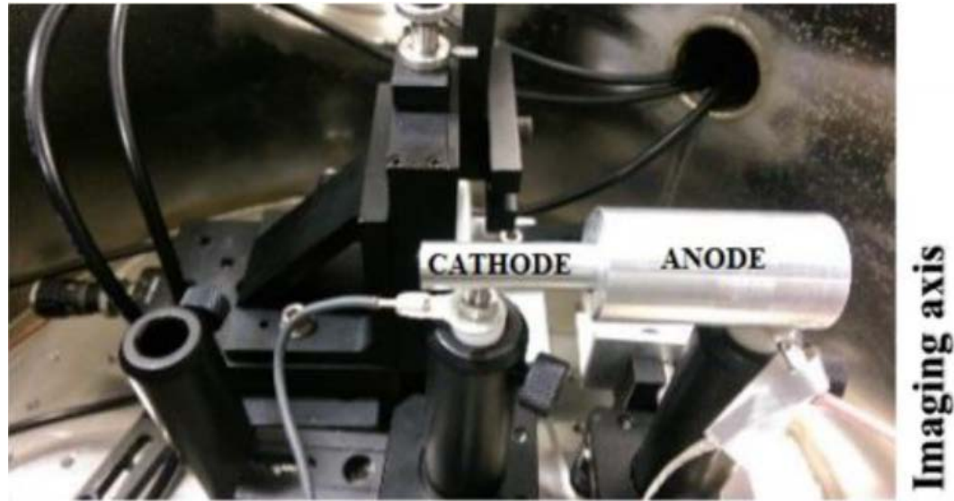
Figure 4: Aluminum coaxial electrodes – attached to 3-D electronic translational mounts
