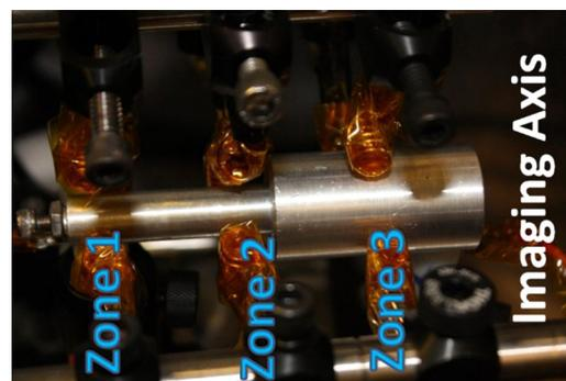
FIG. 1. Coaxial gap experiment with b-dot array zones labeled.
